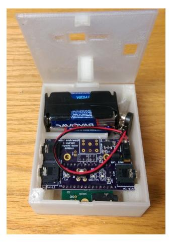
If you want to further seal the box from outside wetness, you can use a rubber block to place in the on/off lid cutout so condensation does not get inside the box. You can also place a small bag of dessicant inside the box to soak up any water condensation.
