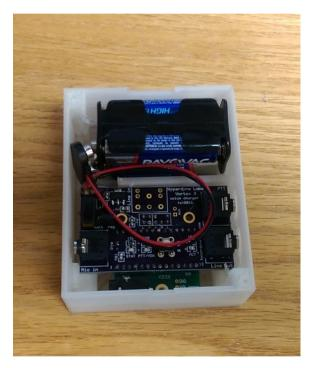
The board will fit inside and secured with the lid. The board is a friction fit and only goes in one way. Holes for 3.5mm cables are on the side of the box.
