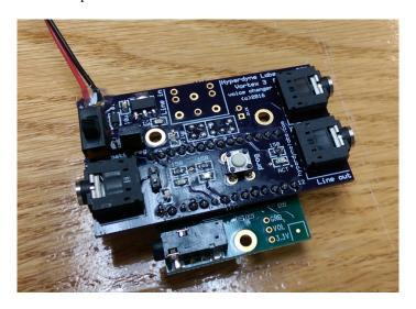
**NOTE:** Handle your board as you would any piece of delicate electronics! Do not get it wet and do not handle it without grounding yourself first! Even a static shock can destroy the delicate components on the board. I suggest when installing the board, insulate it with non-static foam, hot glue, or other material. Handle the board around its edges when moving it. We are not responsible for boards that are rendered useless by improper handling.
