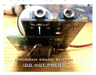
When the board is not powered on, the button has no effect. So if you are changing out processing cards for a different voice effect (and the board is off as it should be) this warning will not apply.
