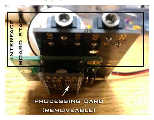
The processing card has female header pins and can be removed from the interface board stack. It is connected via friction fit. This allows you to use other processing cards with different voice effects loaded onto them.
