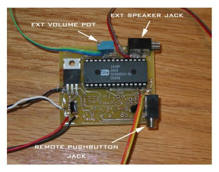
To play out a desired sound, first hook up the remote pushbutton cable to the 1/8" jack shown above. The sound board has 6 sounds that can be played out individually. They are numbered as follows:
