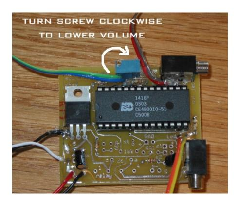
The pot screw **turns 25 times** to go through its entire volume range. So if the volume is too loud going into your external amplifier (sounds distorted), you need to reduce the volume from the sound board.
