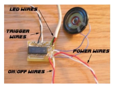
The 2 bottom wires shown coming off the sound board are for the on/off power switch. When these make contact, the board powers up automatically. You can solder these wires to the power switch you plan to use.
