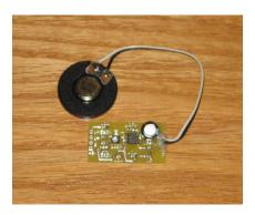
The amp connects to the header on the sound board as shown, creating a board "sandwich":
