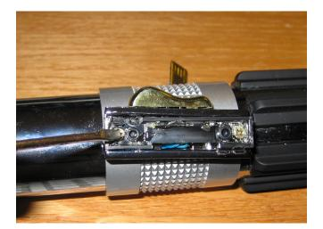
Remove them and the box will come free from the saber hilt. Remove the 2 tiny screws holding the slide switch in place.
