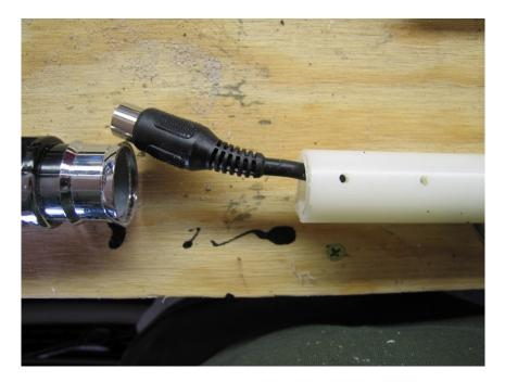
Now line up the drilled holes in the outer and inner tubing. Reclamp the top end of the blade so the holes don't shift between the inner and outer tubes. Insert the blade back into the sleeve and now line up the sleeve and blade holes.
