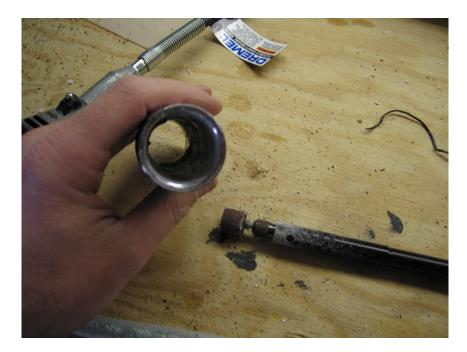
Now fit the outer blade tubing into the sleeve. It will and stop at the raised lip inside the sleeve. Then insert the smaller tubing and line them up.
