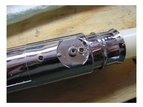
Next you have to cut your tubing so it is 36" long from the emitter opening. Measure from the beginning of the blade (coming out of the emitter) and stop at 36" to the end of the blade tubing. Mark the end of the blade tubing at 36" with a pen or marker. Then remove the blade from the sleeve. Cut off the excess tubing at the end of the blade using a dremel, scroll saw, etc.
