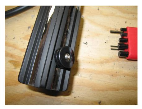
Now drill out the existing hole so it will fit the recharge jack (if you are using our battery system).
