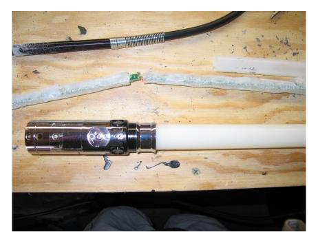
Next clamp the inner and outer tubing at the top of the blade. This will make sure the inner tube doesn't move around when we drill the pilot holes for the cotter pins.
