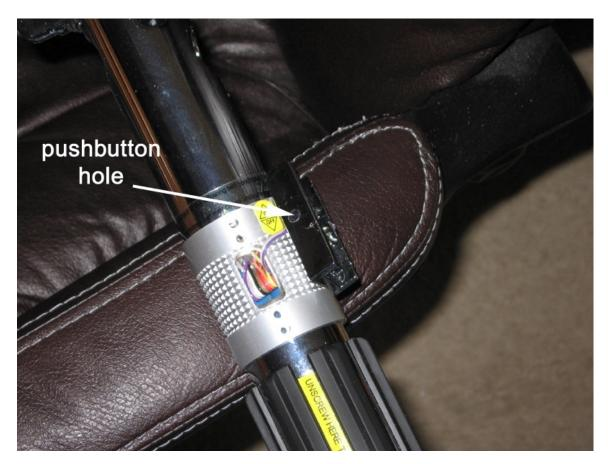
Next make sure you protect the circuit boards with tape or heat shrink wrap. You don't want a bare board inside the hilt, as the metal can short out the board and destroy it!!
