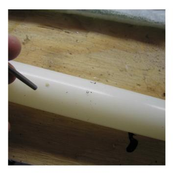
You will drill out the holes further so the cotter pins pass readily through the blade holes.
