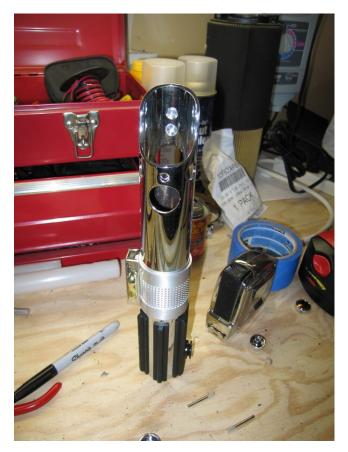
Here the hilt is completely gutted and the inner sleeve has been removed. Save the cotter pins and all screws you removed from the saber.
