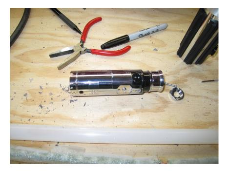
The first step is to see if your tubing fits inside the blade sleeve. If you are using our DuelCore tubing, it may be a bit tight to fit inside the inner sleeve. Thus you will have to dremel out the inside of the sleeve until you can tightly fit the tubing inside.
