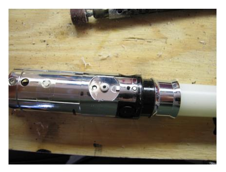
Take the blade sleeve and reinsert it back into the Anakin hilt. It should just slide back down the hilt and you can realign the screw holes.
