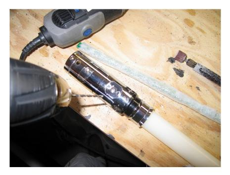
Here is a closeup of the holes drill out. The cotter pins will be used again to secure the blade inside the sleeve.
