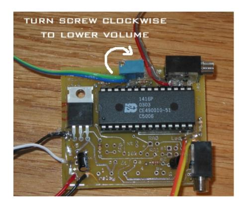
The pot screw **turns 25 times** to go through its entire volume range. So if the volume is too loud going into your external amplifier, you need to reduce the volume from the sound board.
