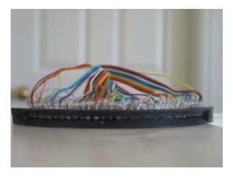
The LEDs were mounted into this original holder and then soldered together. Then the LED assembly was removed from the holder and glued so it retains the same shape and spacing for the LEDs. You can make your own LED holder or simply glue the LED assembly right to the visor area if you like.
