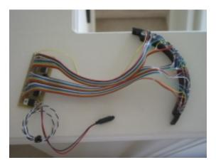
The circuit will run off a 9V battery or a 6AA batt pack. The wig wag sequence lights 3 LEDs across the LED array at a speed that was taken from some of the BSG cylon scenes.
