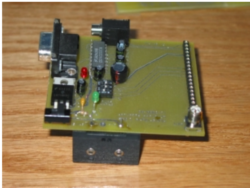
Base station board
