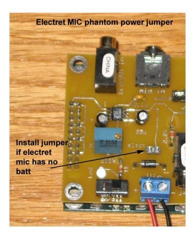
NOTE: A condenser mic will not work with the board, as the output will be too low for you to hear.
