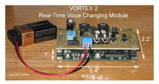
The dimensions of the Vortex 2 module are (not including battery or cables): 3.4" L x 2.2" W x 1" H.
