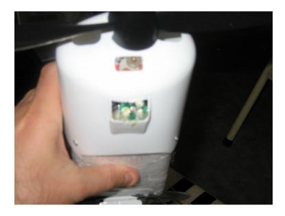
Next install the processor board and plug in the LED ribbon cable to the header on the board. The ribbon cable should be facing away from the board if it is plugged in correctly.
