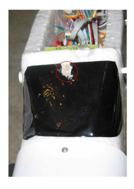
This LED comes on when you press the X-port button on your transmitter, so you have some feedback that the circuit is working. It will also blink every 5 sec as a heartbeat.
