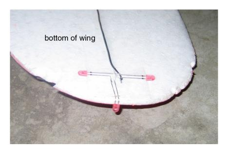
Use packing tape to secure the wing clusters and cover up the exposed leads.
