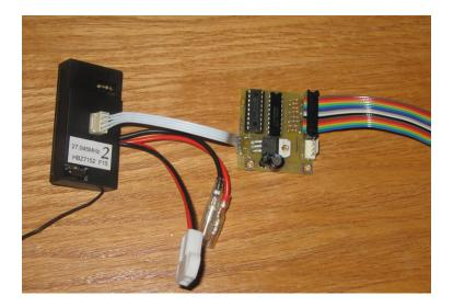
The light processor board also has an X-port male "passthrough" connector. Take the Super Cub X-port extension cable that runs down the battery box (this is the cable that is normally plugged into the stock receiver) and plug it into the male header on the processor board.
