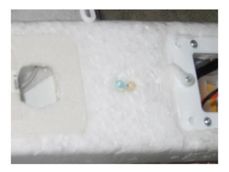
You can use a dab of hot glue to hold the LED in place. NOTE: Point the LED towards the back of the plane and slightly down so you will be able to see it when the plane is flying away from you.
