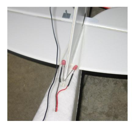
Next install the two fuselage lights. It doesn't matter which side the yellow or green resides on, it depends on your flying preference. We found it works well with the green on the right side of the fuselage (looking from the front).
