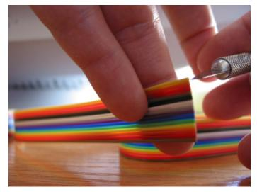
Then splice all the wires using some wire cutters/splicers. The wire is thin so don't use too much force when splicing.
