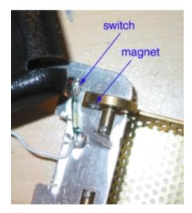
13) You may have to cut a larger notch out of the comm. halves and the midplate in order to fit the magnet. The magnet should ride on one of the wheels and be able to pass through the midplate and the comm. shells without any impedance. Most of the roddenberry.com kits will need extra filing on the midplate and the comm. halves in order to have the magnet pass through without "catching".
