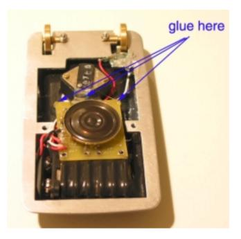
**10**) After the glue has dried, try to refit the bottom comm. half onto the midplate. The bottom should still fit with a small gap (or no gap). You can attempt to position the battery better to MINIMIZE the gap on the lower shell half. Not to worry, a small gap will be typical, but it will disappear once you screw
