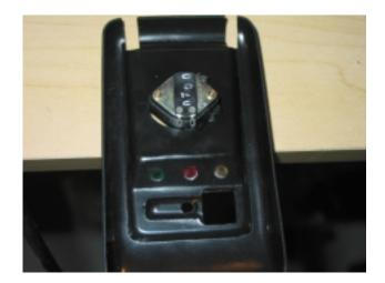
3) Now retest the comm. fitting by taking the 2 shells again (with the midplate) and trying to close them flush (as if you were assembling the comm.). The motor should sit up a small amount from the front of the comm. shell, and the 2 shells should now sit flush on the midplate (so you can close up the comm. later without problems).
