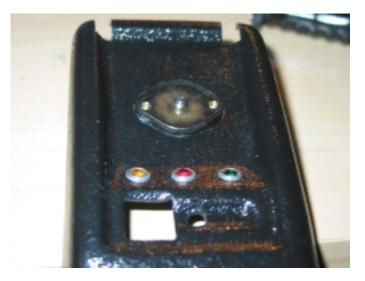
4) Hot glue the motor from the inside of the top comm. shell. If you hot glue the black plastic sheath that the motor is housed in, then you will be able to fine tune the motor's position. This is because the sheath moves up and down on the motor, which will provide you with some leeway. Here is a picture of the glued down motor. You can also see the properly drilled holes for the backlit jewels and the middle knob hole.
