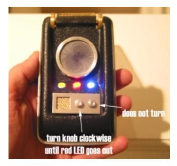
Here is a table of comm. features based on how long the knob is held in place (the red LED is unlit):
