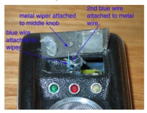
34) Test fit the com plate onto the top comm. half. You should be able to twist the button clockwise a small amount to make the "wiper" contact the other wire. The red LED will extinguish each time you make contact. TAKE YOUR TIME and tweak the working of the knob so it is reliable. It just takes some proper positioning to get right. The wires are also delicate, so the less you bend the better the install will go.
