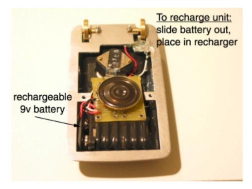
All you have to do is carefully slide out the 9V battery (it slides out easiest if you pull toward the bottom of the communicator. Carefully unhook the 9V snap connector. Now take the battery and place it in the included recharger. The recharging should take about 6-12 hours for the low trickle charger included. Please read the instructions included with the recharger!
