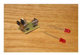
The tilt switch is installed so when the unit is on its side it will come on automatically. The unit can run off 2 or 3 watch batteries (model 357). There are also 4 different sequencing/pinging modes on the board.
