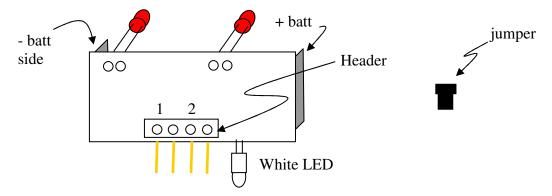
The header is shown in the above picture. 2 pins are labeled "1" and the other 2 pins are labeled "2. Use the included jumper connectors to choose the mode you want by shorting the pins per the below diagram.
