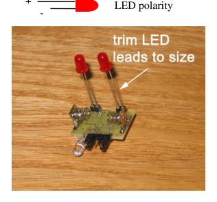
The included LEDs are super bright red 5mm LEDs. You can replace them with any color LEDs that will work off 4V. This includes yellow, green and some lower power blue LEDs.
