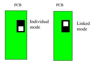
You can also connect 2 wires to the pads next to the mode switch if you want to remotely control the mode selection parameter. These wires can be connected to another remote switch so you can choose between individual and linked mode without using the onboard slide switch. The hookup is the same as the switch inputs. When you short the 2 wires then this activates individual mode. *Note: If you do this you will want to set the slide switch to the linked mode position and keep it there!!*
