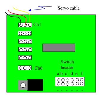
The board also has a 12-pin header that is used to wire up the external switches that control each servo. The header is labeled with the pin numbers corresponding to the servo it controls. The top row of the header is the switch input for each channel, labeled a to f (a=ch1, b=2, c=3, ...).
