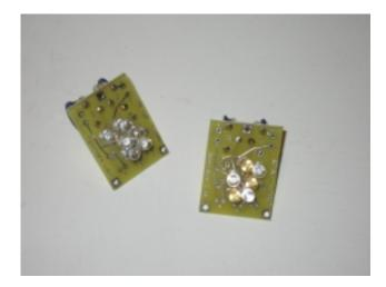
These boards hold several LEDs for each color (blue and red on one board, green and yellow on the other board) in a honeycomb-type array. This maximizes brightness and maintains a uniform brightness over a given area.
