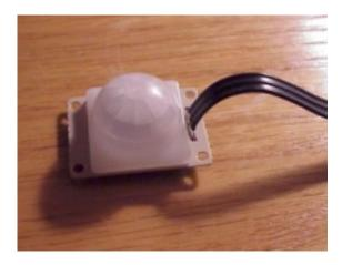
The IR sensor derives power from the sound board. When the sound board is powered up, it will take the IR sensor a maximum of 30 seconds before it responds to any motion. This is its warm up period. After that, it will activate the sound board if any motion is detected in its field of view.
