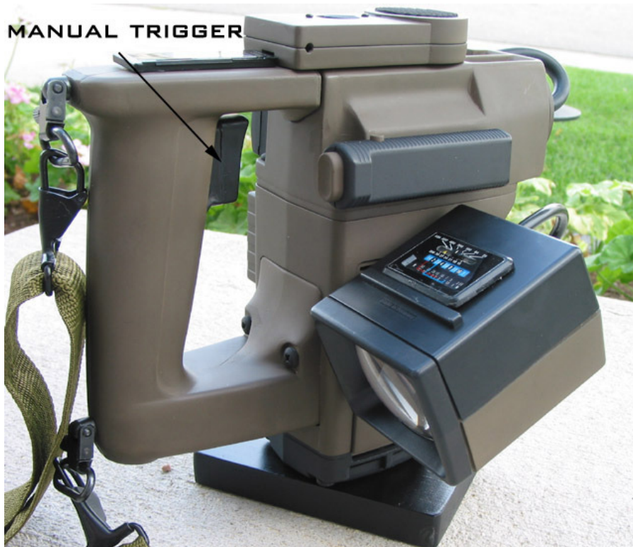
Here is the LCD and sound kit installed in a replica motion tracker.
