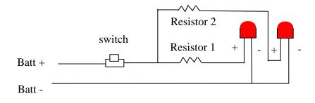
The resistor value you should for each LED comes from the first table! This is because you are hooking up each LED to the battery in a parallel configuration, which is just an extension of the first figure.
