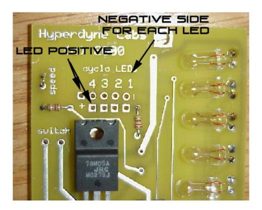
The assembled boards have a header already installed on the board where the LED connections go. You hook up the included cable so you can easily run the wires down to the cyclotron area. When you plug in the cable, each pair of 2 wires are used to connect up each LED.
