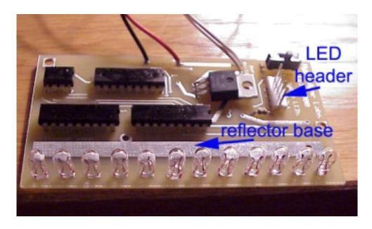
The 2 switch wires coming off the board are connected up to the master on/off power switch. This allows you to keep the batteries connected, but you can turn the unit on and off by just using the switch.
