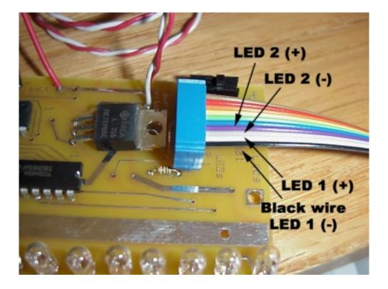
The first black wire is the (-) lead for LED1, the next white wire is the (+) lead for LED1. The next pair or colored wires are for LED2, the next for LED3, and finally for the 4<sup>th</sup> LED. Note, the last 2 wires are unused.
